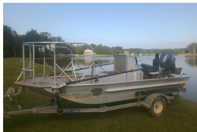
Electrofishing equipment was used to collect a fish sample from Swan Lake, July 2022.
